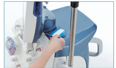
A patient card that can record prescription data and the results of three treatments.
